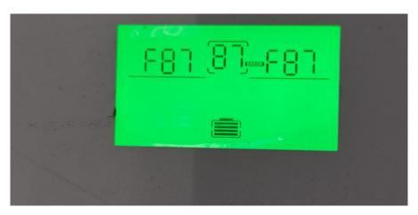
After our lab simulation test, If the short circuit cap is not installed in the control board on the right, will result in 【87】. Therefore, you can use the steps below to solve fault 【87】 short circuit cap
