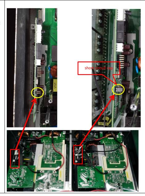
Through the above steps to check on the right side of the control board short-circuit cap good after installation, please plug in the battery whether boot validation will quote [87] the ERROR, if the problem remains, please contact your installer.
